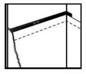
Hook fixtures on rail and slide into position. Attach hanger wires.
